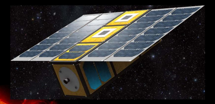
\* Shown with DSI COMET-1 Water Thruster Integrated. Flight articles used will incorporate Reflectarray Rectennas (combination solar/receive & transmit antennas).
