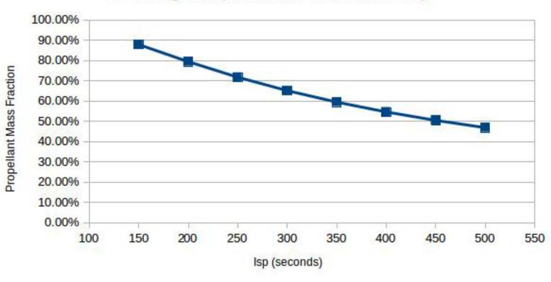
Second Stage: Propellant Mass Fraction Vs. Isp
